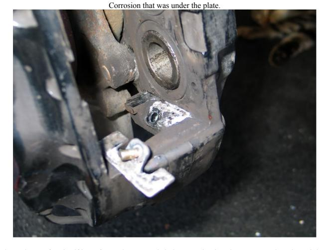
Back of plate. Plate surface itself is perfect and not corroded, the corrosion is only on top, stuck to the stainless, only the aluminium is corroded. These plates clean up beautifully with a wire brush.
