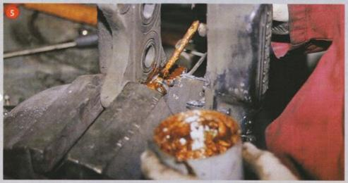
Once you're happy with the condition of the surface, use a brush to spread a very thin coat of high-temperature copper grease around the area that the plate will sit on. Don't overdo it, though; you don't want grease finding its way onto the pads and discs. This will go some way to prevent corrosion recurring. Eventually, though, this will dry up and corrosion will set in again. You're looking at up to five or even 10 years, though
