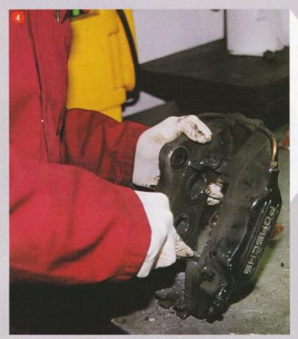
Although the plate must be replaced, the caliper itself can almost always be reclaimed for another tour of duty. You'll need a fine file carefully to smooth off any corrosion in the area round the stainless-steel plate. It's important not to get too carried away, though, and remove good metal from the caliper, otherwise the pads won't be held firmly and could vibrate and squeal. Check that the new plate sits correctly
