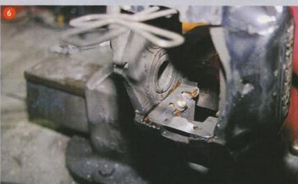
Now you can fit the new plates. It's essential to use thread-locking compound on the screw threads. Always use new plates and new screws; they come together in a special kit. Wipe off any excess grease at this stage
