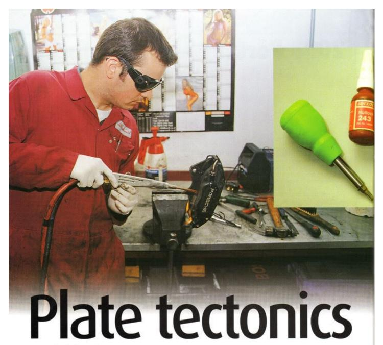
Light-alloy brake calipers – as fitted to many Porsches during the 1980s and 1990s – can suffer from corrosion, which makes it difficult, if not impossible, to fit new friction pads, and can cause other problems, too. But renovating them isn't a particularly difficult job, reckons Philip Raby. Photographs by the author and Peter Robain
