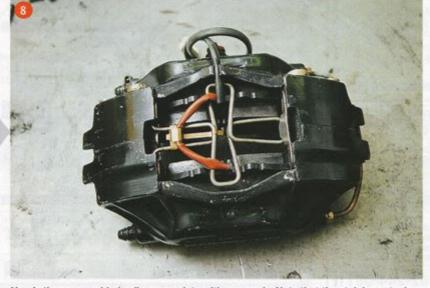
Here's the reassembled caliper complete with new pads. Note that the stainless-steel plate now sits firmly against the aluminium. The caliper shouldn't require any further attention – apart from routine fitting of new friction pads as required – for several years
