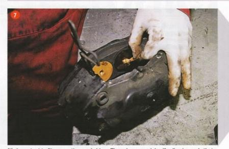
It's important to fit new anti-squeal shims. These have special self-adhesive pads that stick to the backs of the brake pads (so remember to peel off the backing paper before fitting the pads). The shims dampen any vibration, thus reducing the risk of noise during heavy or even moderate braking. Tit new wear-indicator wires and clips, too
