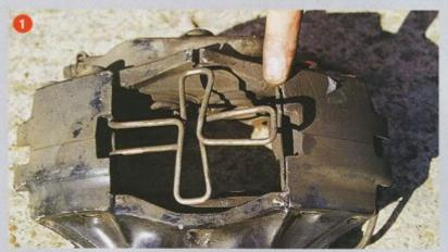
This is a front caliper from our 964-model 911 Carrera 4. The stainless-steel plate on the left of the photo has clearly lifted away from the aluminium caliper body beneath. It would be impossible to fit new brake pads in this situation without grinding material from the pads' backing plates – which certainly isn't recommended
