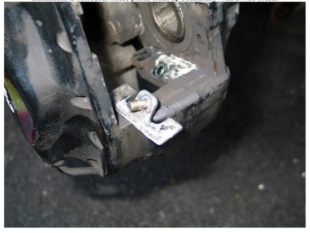
Back together. Fresh black is the new paint and you can see the 'coppa slip' coming out from under the plate. You can also see the plastic mallet used to persuade the disc off, worked very well without any damage.
