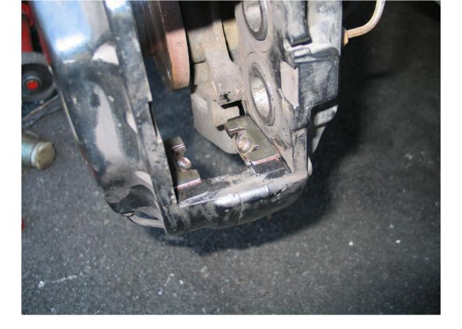
Another finished view. The plates came up like new with a gentle application of a wire brush. These plates are actually the top ones swapped over with the bottom ones.
