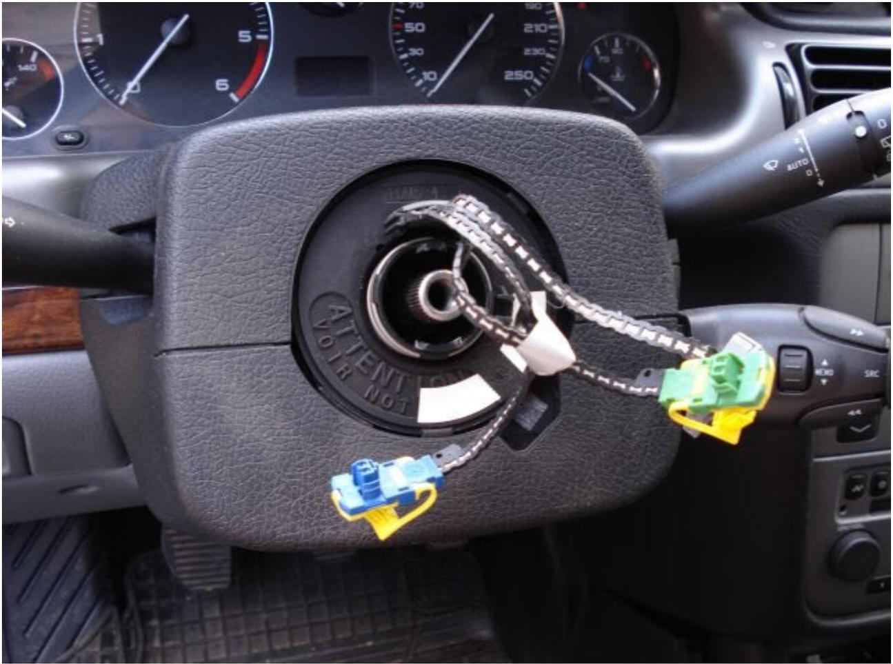
Now it's time to remove the cowling (hey, it's easier to leave it until now, ok?) Two screws (that's quite a reach up inside TBH, too long for my 'ickle set so I used a my flat bladed screwdriver 'cos it fitted in the screws)
