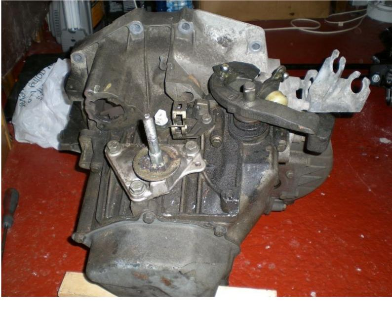
First job on the gearbox is to change this collar which the release bearing moves along.
