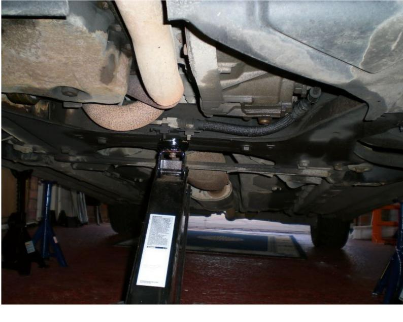
IMPORTANT!!!! Support the engine NOW with a bit of wood on a jack but don't raise the engine.
