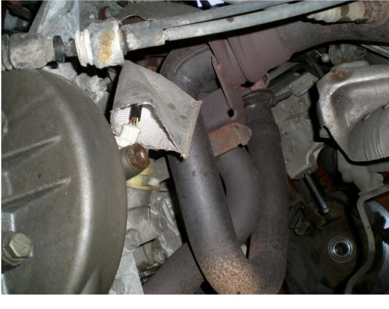
Up top, you should be able to see some wiring looms on a plate attached to the side of the gearbox by a big bolt right in the middle of this picture. This is the engine earth, and you'll want to clean up the plate, starter earth, and (once the box is out) the gearbox here.
