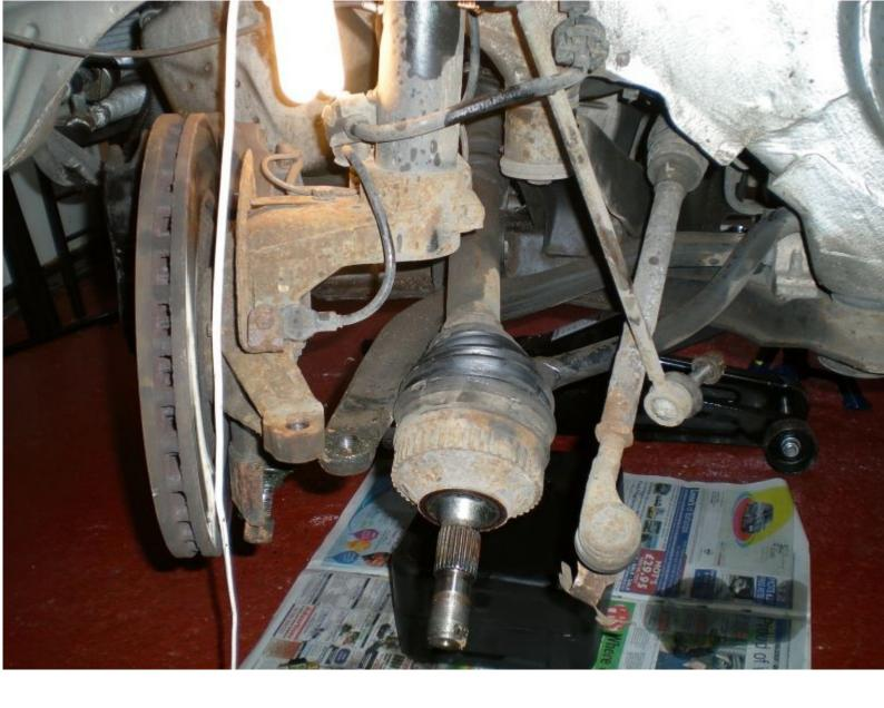
Take a well-earned break then remove the n/s driveshaft by simply pulling it. Inspect the gaiters for splits as they're MOT failure points
