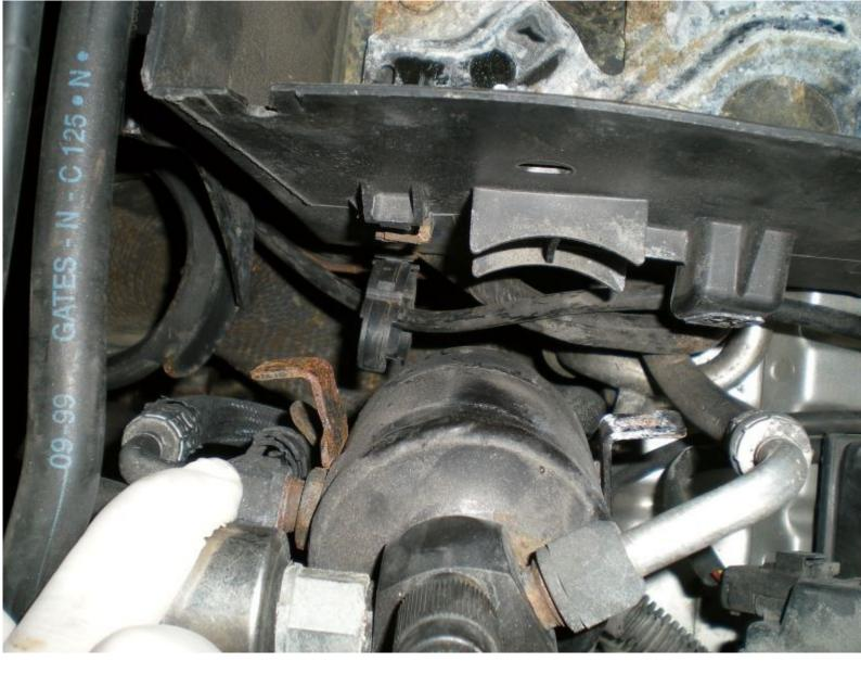
With the battery box out the way you can do some preventative maintenance if you want. Remove and clean up the main earth connection (shown to the right of the picture under the light connector), and check the wires are un-corroded and firmly in the battery clamp. I ended up cutting, stripping and re-attaching both wires.
