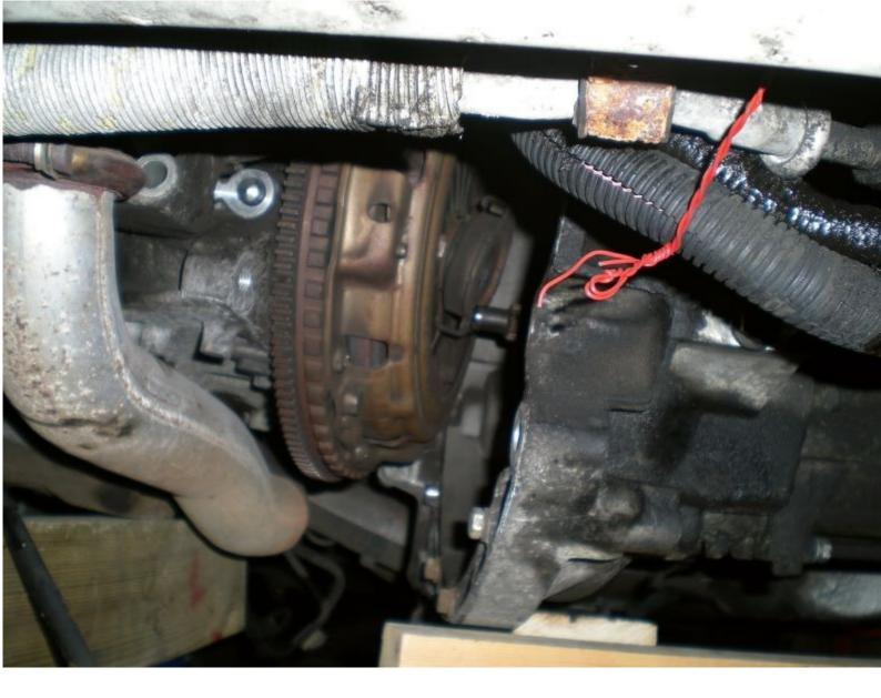
Expect the engine to want to rotate. This can lead to whoopsies like this. Also note that the holder for the Pin Of Evil makes a nice carrying handle if you wedge the handle of a breaker bar in it!!! Just be careful not to pull your brake wear cable like this. You can see how the gearbox has caused the jack to put a hole in my garage floor Fit's HEAVY!!!
