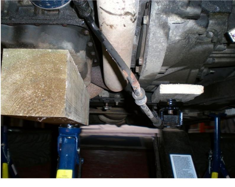
Up on top is the gearbox mounting. Take the large nut off then undo the 2 torx bolts to get the mount free.
