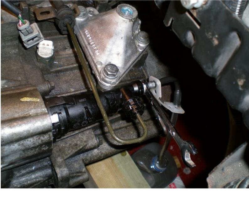
When bleeding, you want to either have the nearside jacked about 1-2 foot higher than the offside, or do this after EVERY pump of the pedal otherwise you'll just take in air due to the ridiculous design of the reservoir.
