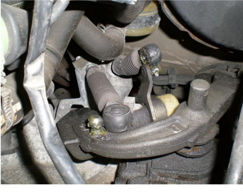
One 10mm bolt is all that's holding the flywheel sensor in. I strongly recommend you tie it up somewhere as it has a habit of falling around and catching on stuff
