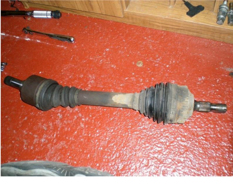
We can't remove the o/s driveshaft yet because it's held into the intermediate bearing (part of the lower engine mount), and the nuts to remove it are as good as inaccessible on the ES9J4 due to the 3 exhaust pipes in the way (may not be the case on the ES9J4S). So considering the subframe needs to come out to get the gearbox out, lets take it off.
