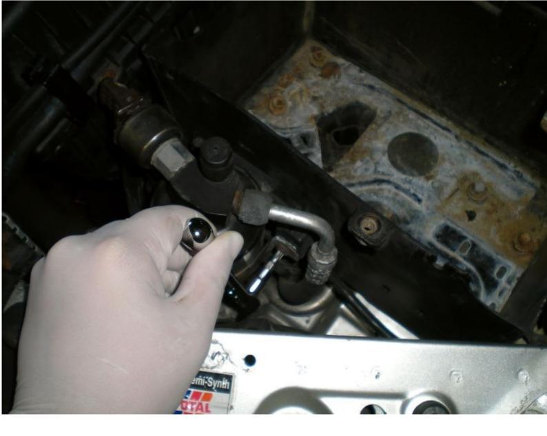
then pull the unit out slightly before sliding it to the right to unclip it. There's some wiring behind here you'll need to unclip
