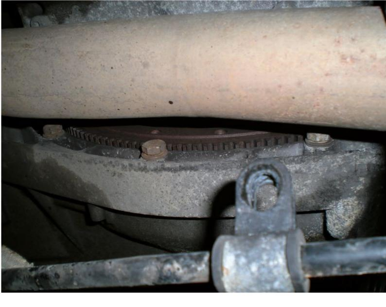
While you're under here, I'm going to show you the hidden gearbox bolt. It's in the middle of the picture, with the gearbox at the bottom and the sump visible at the top. This one isn't obvious because it goes from the engine into the gearbox whereas the others are the other way around. Don't undo it yet.
