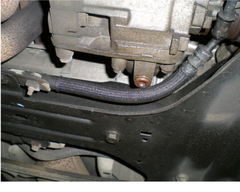
Here's the key you'll need to undo it with. 8mm square. I find it best to ignore the hole going through it and slap a ring spanner on the other end.
