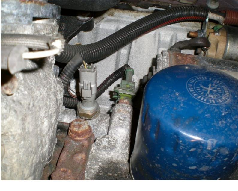
You can then use a flathead screwdriver to get the starter clear of the bell housing.
