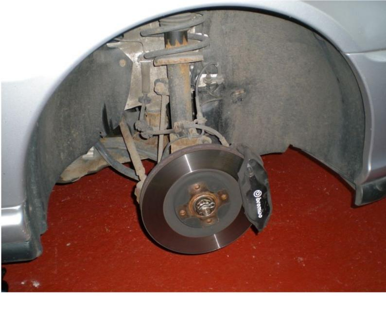
Put the wheels back on (don't bother with the locking wheel nuts), put the car back on the floor and use your 35mm socket and breaker bar to take the paint off your alloys Be careful about that... Chances are you'll need to stand/jump on the breaker bar
