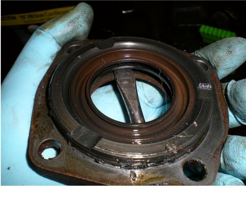
May as well clean up some of the muck from the gearbox while you can using some heavy duty engine degreaser. Note I've not gone mad with it, I've avoided seams and I've DEFINITELY avoided the gear selector's moving bits! You do not want degreaser inside your gearbox!
