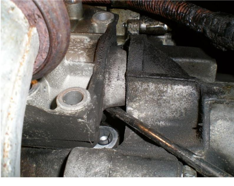
While you're down here, there's 3 small bolts holding a little cover onto the bottom of the bell housing next to the exhaust pipe.
