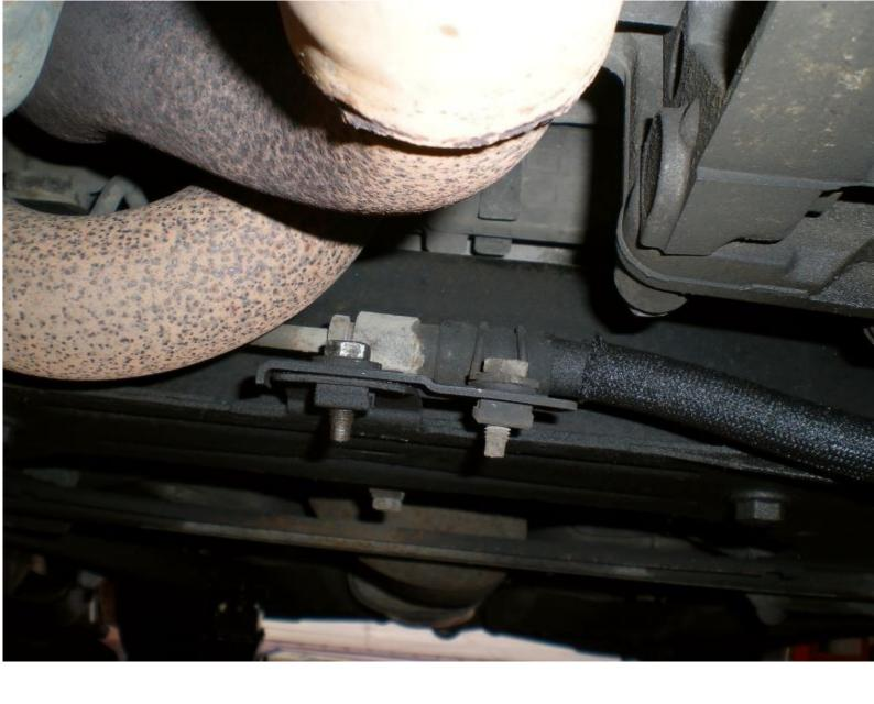
Unbolt the pipe from the gearbox too. There's 2 bolts to undo, the one at the front I've already removed in this picture.
