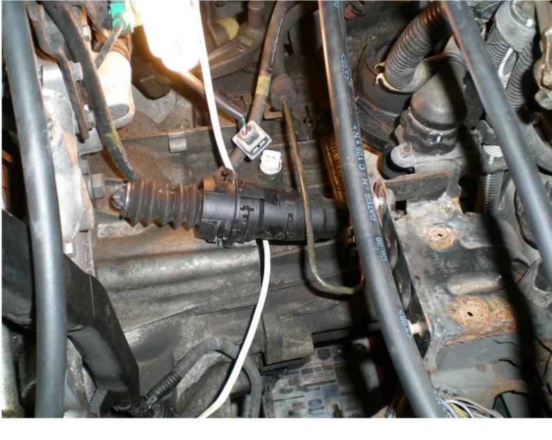
If you get back under the car and look behind the gearbox you should see something like this. Under the heat-resistant "bag" is the connector for the speed sensor. Pull him out.
