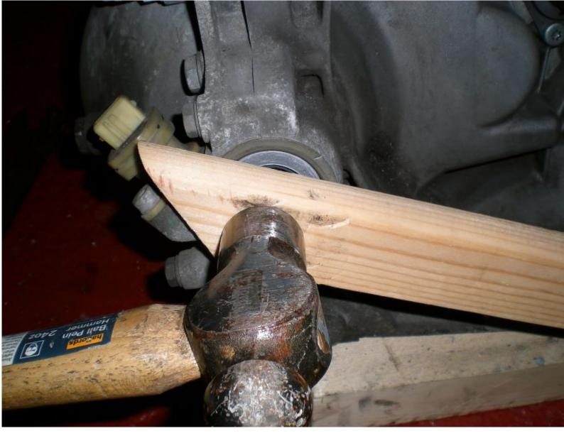
Unbolt the n/s diff seal holder (the red bit) from the other side of the diff. (sorry, didn't take a picture of this with the box off the car (\*\*)
