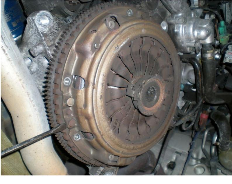
One flywheel. You should clean this with brake cleaner. Note there's 2 sets of teeth around the edge. The fine teeth are for the starter and the fat ones are for the flywheel sensor
