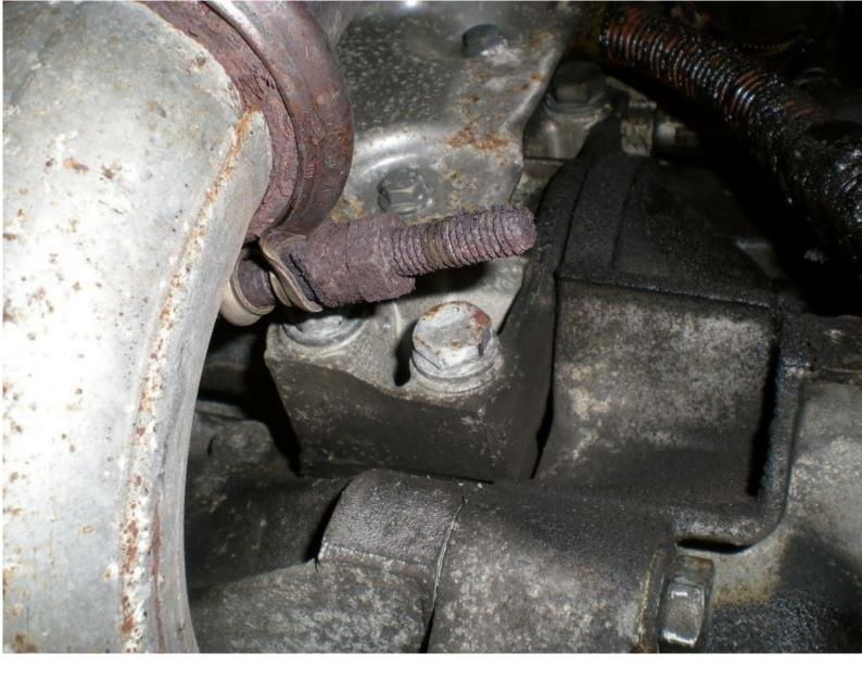
Without the shield, you can see the 3 bolts holding the starter in place - 1 at the top, 2 at the bottom.
