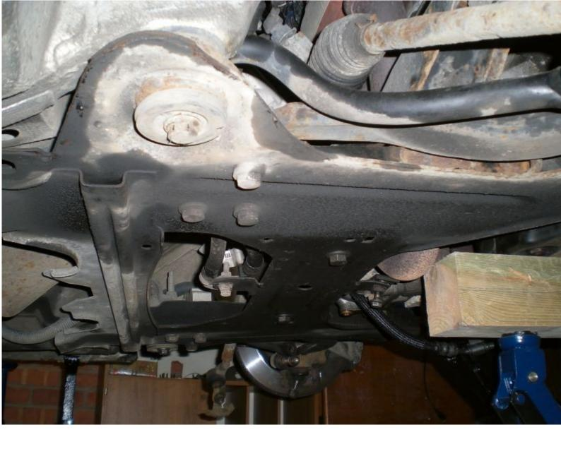
To the back of the main subframe bit (behind the steering rack) are these pipes held on by a nut+bolt. Undo to free the pipes.
