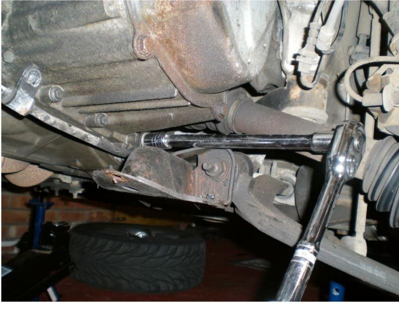
Here's the gearbox oil drain plug.
