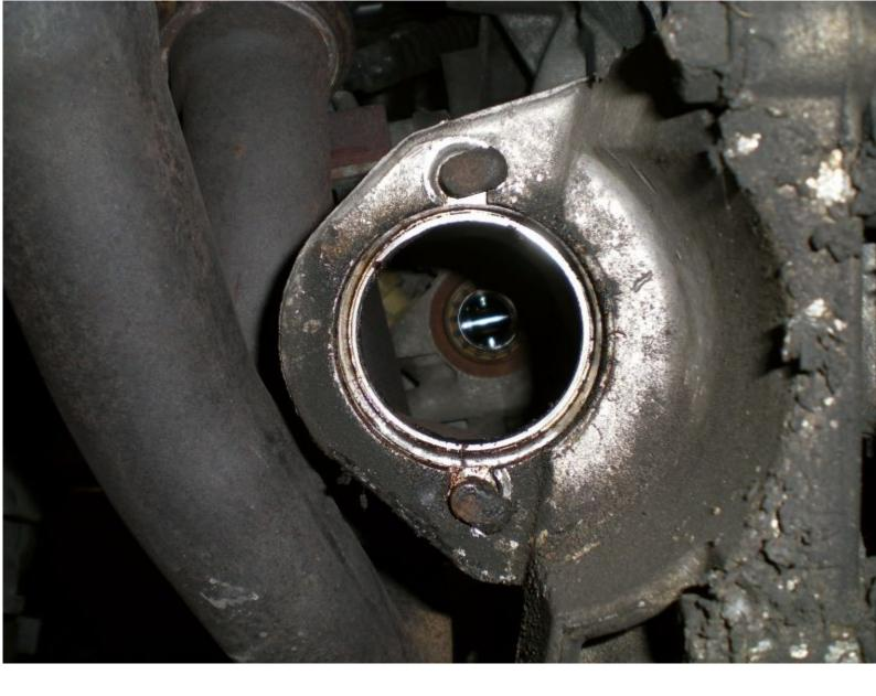
This is what you're fighting here, and without the subframe in the way a small 1/4" ratchet should have no problems getting in. Try not to damage the heat shield. It may be an idea to order a new one first since it's pretty brittle, but I put my old one back on later with a few big washers...
