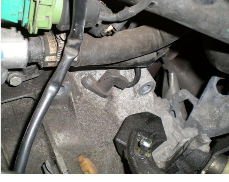
D9: The clutch slave cylinder has to come out now. This is not fun. Firstly free up as much of the pipework as you can. To remove it, you push it inwards and turn about 45 degrees anticlockwise. As you can see, I bent my pipe a bit Alternatively you can pull the steel clip that's holding the pipe in half-out and pull the pipe out. It'll be VERY messy though, and brake fluid's evil stuff.
