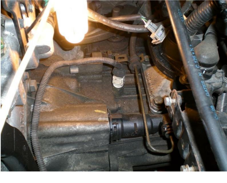
Here's the gear linkage balljoints. Just get a flat screwdriver under them and pop 'em off.
