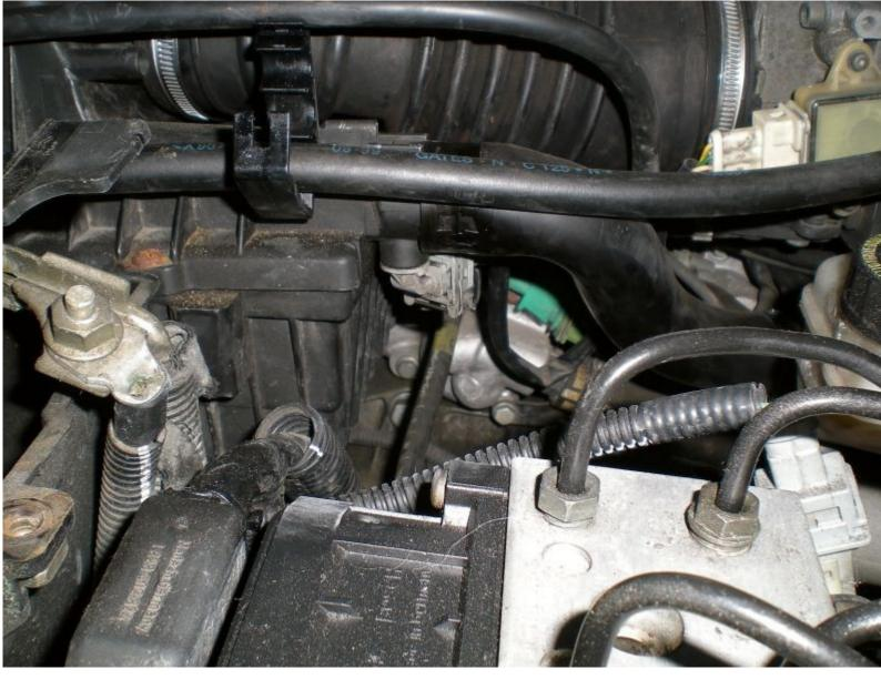
Unclip the hoses from the air filter box along with the large rubber hose...
