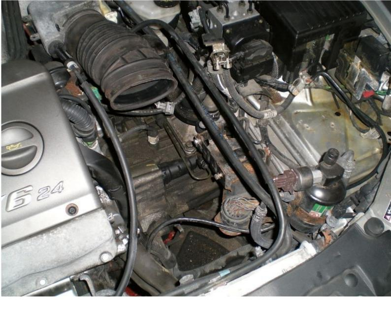
You want to remove the main air hose now by unscrewing the huge jubilee clip then pulling it out. Be careful as there's a push-fit joint into the engine on the left hand side as you're looking at it
