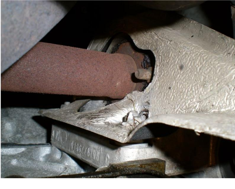
The o/s driveshaft should now pull out. Again, check for splits.
