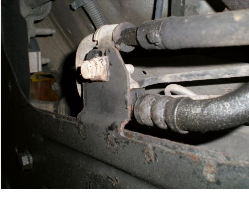
Remember the bolts under the steering rack? Undo them now. There's large ceramic washers between the rack and subframe, so catch these before they end up falling in your gob
