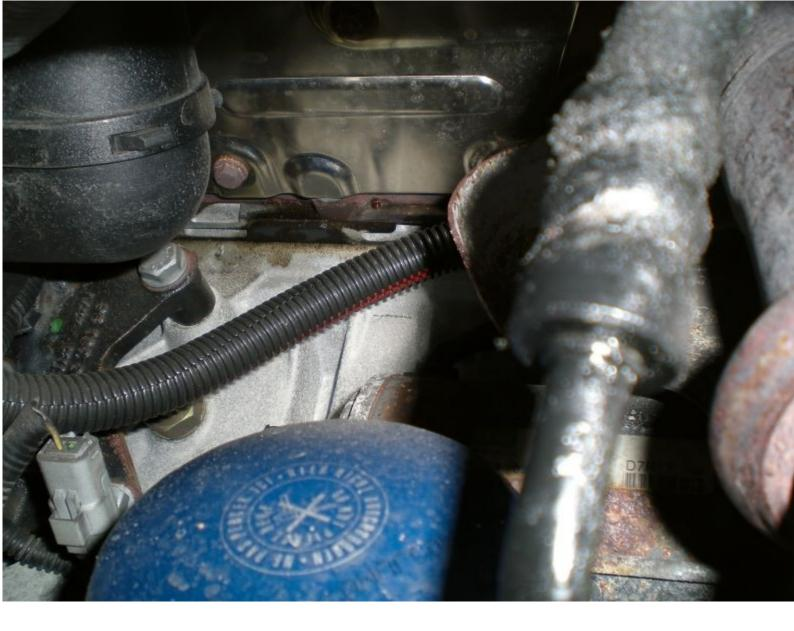
Getting to it isn't obvious. First, if your exhaust pipe clip's in a dumb place like mine was, slacken it, move it round the front, then re-tighten it. The 2 smaller bolts you can see at the top hold the heat shield on. Get 'em out.
