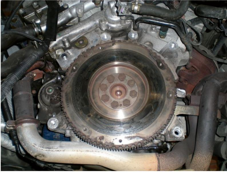
Fit the new clutch friction and pressure plates. The friction plate needs to be PERFECTLY in the centre. There's several ways you can do this, but be aware your average clutch alignment tool won't work.
