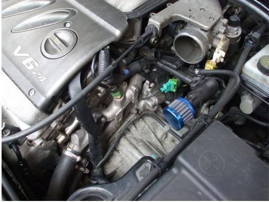
I started with taking the two bolts out of the cable holder at the front of the engine because there is a 10mm Thermostat casing bolt UNDERNEATH this cable holder.
