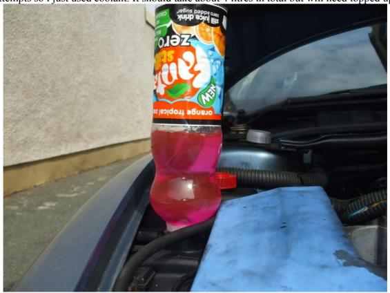
Place the bottle in and fill. Then start your engine. I had the GF sit in the car and hold it at 2000rpm. You will see the bubbles coming already! Rush to the front of the car and open the Radiator bleed point by a quarter turn. Nothing should come out straight away. Wait until it does come out and runs free of air. Now shut it and move to the bleed point above the heater matrix!
