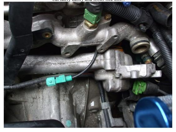
Once off inspect the casing and clean if necesary. Mine had bits of rust like debris in it. The Thermostat will take a bit off riving to get off. I used a flat screwdriver and dug it into the seal. It did damage it a bit but don't worry about that. Don't be too rough though in case you Thermostat is OK and can be re-used. The inside of the casing with the Thermostat out looks
