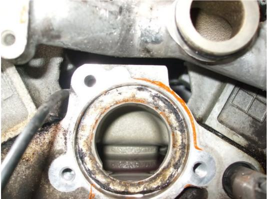
I gave both sides a good clean and where the seal sits a very thin coat of liquid gasket....
