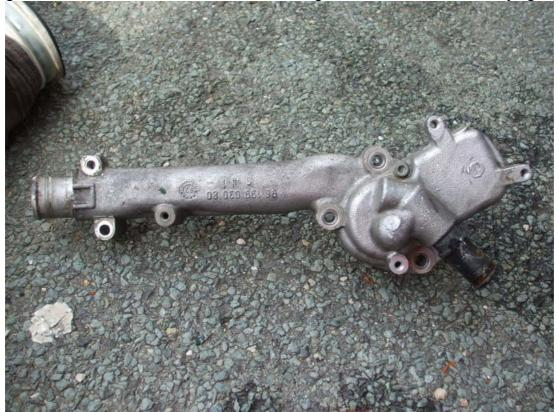
There is however, a black bar on the underside of the Thermo casing towards the back of the engine. It holds a bar on. I bent mine back with a screwdriver. Its important to get this off as on of the main bolts that holds the casing on, is UNDERNEATH this. So it has to come off!
