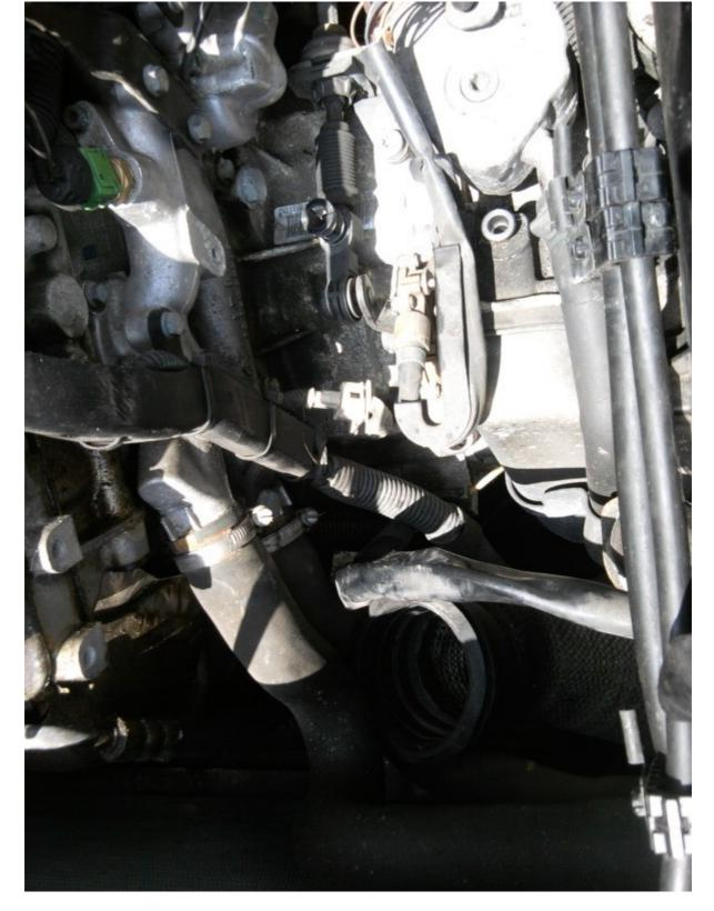
You will see a small blue cap - pop this out (and catch it!) and also remove the dipstick. Be sure to clear all loose debris away before you do this. This allows more air to get in the box while you are draining.
