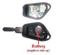
Note the position of the batteries (negative side up), replace with two CR 1620 3volt batteries.
