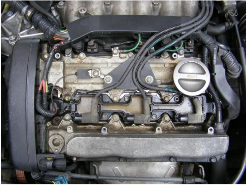
This is the breather that needs to be removed using the long nosed pliers. you need to squeeze the ridge are on the top & the bottom & it should, with a bit of a wiggle, come off. Be very careful as this plastic can be brittle & break easily:
