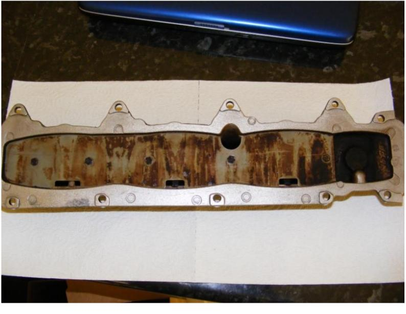
I used Loctite 5980 (it's what Pug use) as sealant. It's perfect for your oil sump too. It's not the prettiest of jobs to do, but make sure you've got a reasonable amount on there, following the path of the sealant you removed. You need to make sure the sealant is higher than the surface of the metal casing as it will squash when you bolt it back down:
