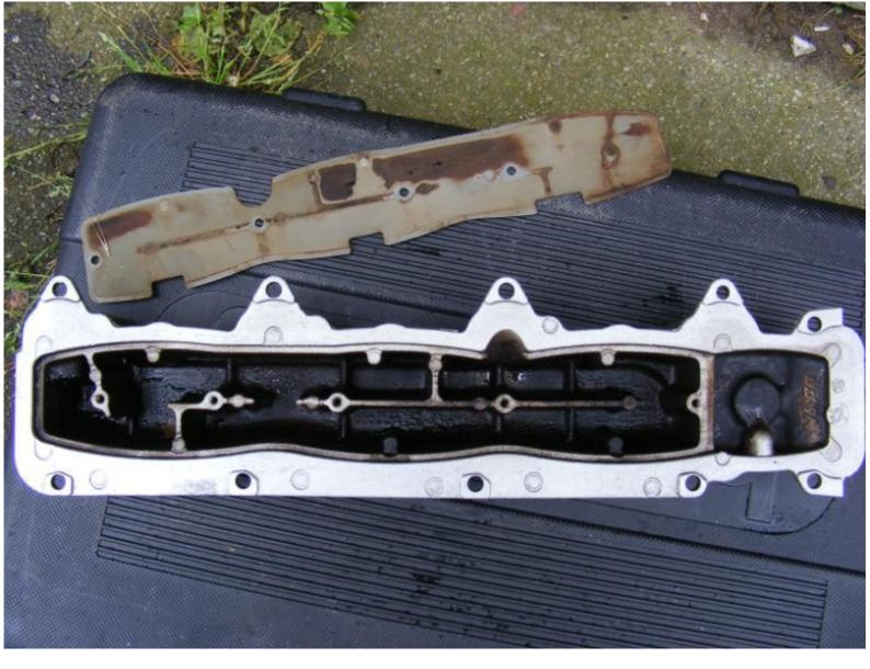
You'll also need to degrease the top of the engine where the rocker cover goes. Obviously you can't brush GUNK on there, so I dipped the cloth into the bowl of GUNK & just kept wiping away, then cleaning off till it was grease free.
