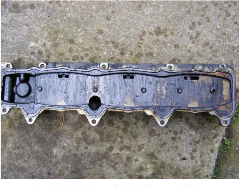
Remove the  $5 \times 5$ mm bolts & you have this. Now is the time to remove the old sealant:
