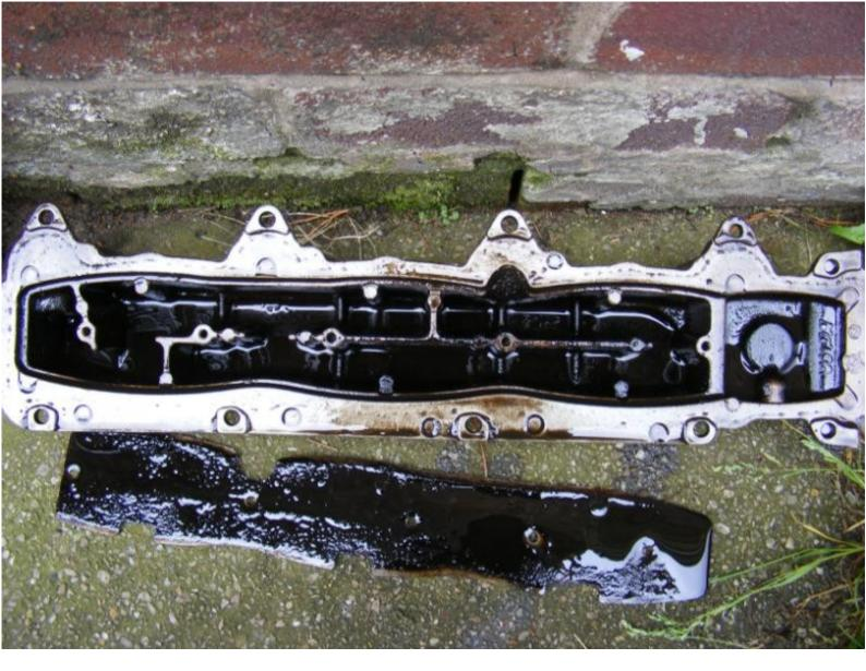
Use your wire brush to remove all the old traces of sealant, it doesn't take long. I then poured some of my brush on GUNK into a bowl & used a paintbrush to apply it around the edge of the rocker cover & both sides of the metal plate you removed above, I repeated this a couple of times. Leave for 10 mins then rinse off, I used the outside tap, it was a lot faster:
