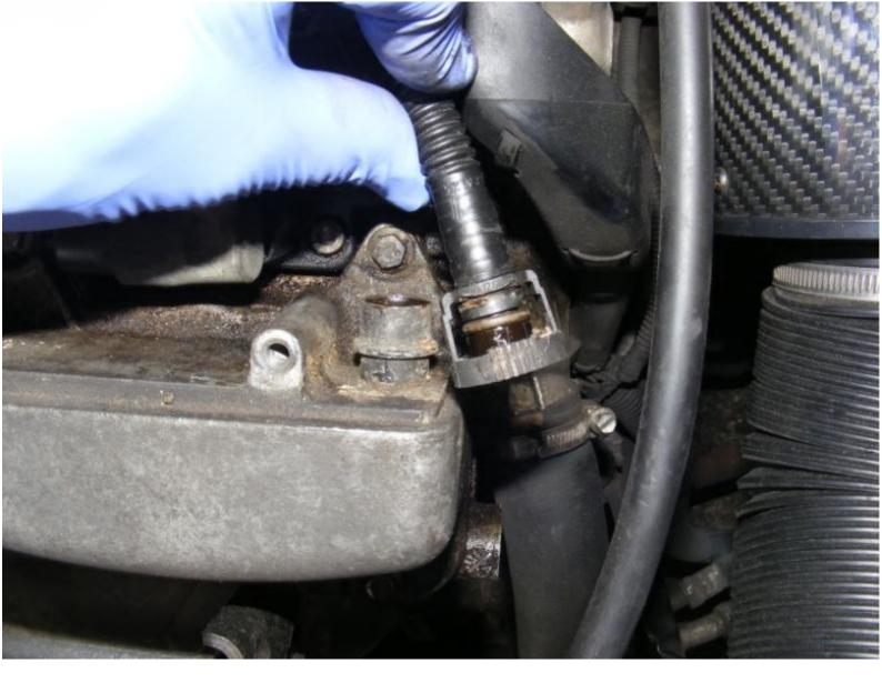
Next, you need to disconnect the power feed for the coil pack, it's the large plug here alredy removed. You also need to carefully unclip the wiring harness from the cam cover by pulling it to the right:
