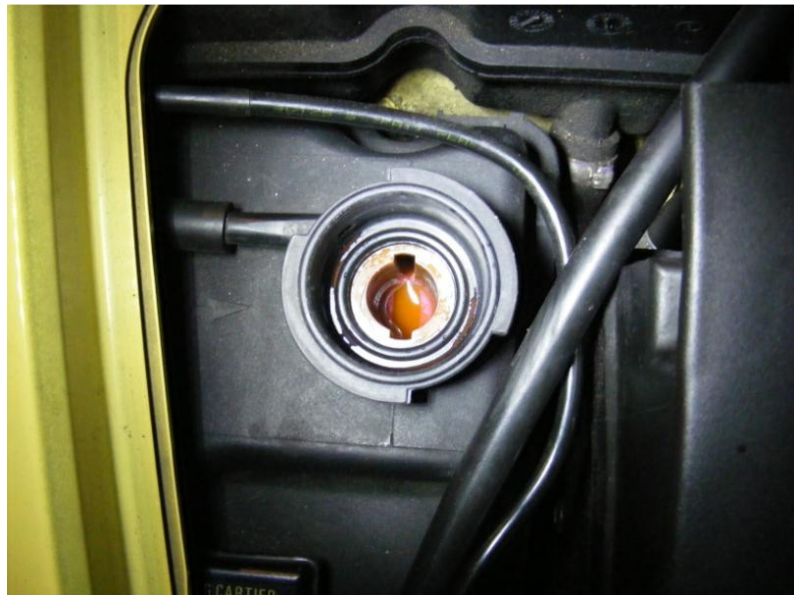
Brake fluid reservoir: (markings are rough)
