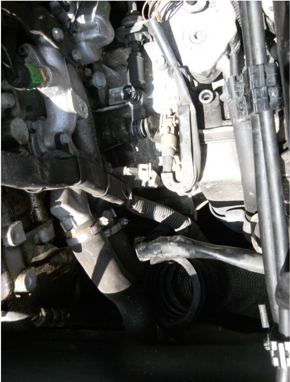
You will see a small blue cap - pop this out (and catch it!) and also remove the dipstick. Be sure to clear all loose debris away before you do this. This allows more air to get in the box while you are draining.
