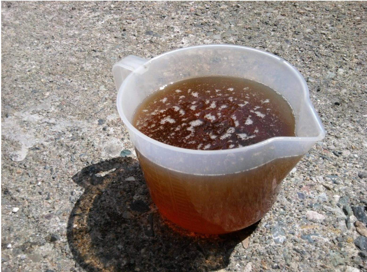
Refit the dipstick and the blue plug, fire up the car and let it heat up again, then repeat the above. It was at the third flush that I saw the oil getting clearer -I used the whole 20 litres too for good measure..
