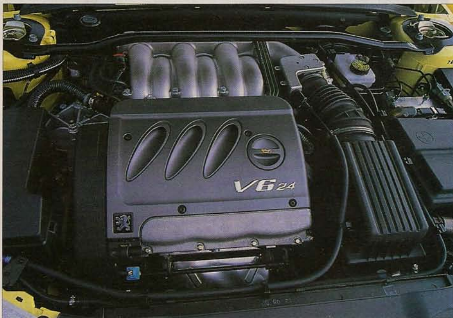
Smooth, lusty 24-valve V6 is the new Citroën/Peugeot/Renault unit. Powers the Coupé from 0-60mph in 7.3secs
